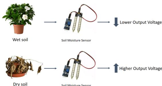
**Fig. 4: Soil moisture sensor module**
