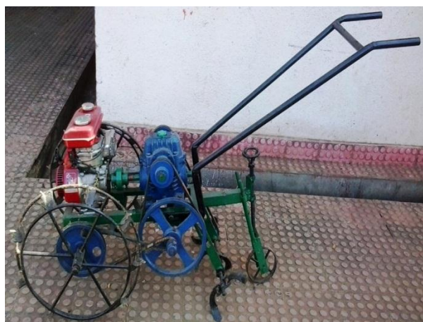
Fig. 3: Power operated rotary weeder
