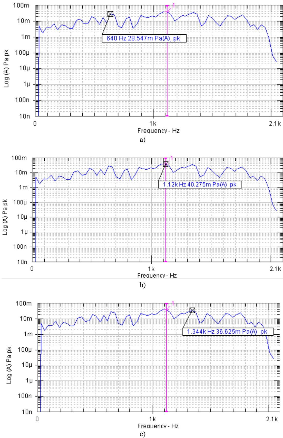
Fig. 2: Spectra image of a) Immature coconut, b) Matured coconut and c) Over-matured coconut
