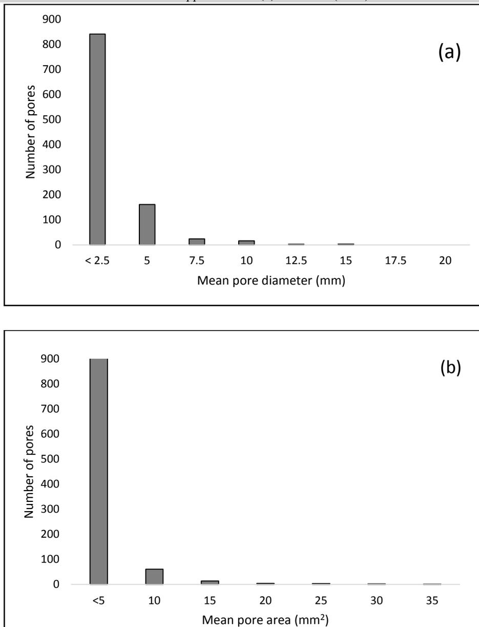
**Fig. 6: Pore size distribution in bread crumb: (a) Number of pores as a function of mean pore diameter. (b) Number of pores as a function of mean pore area**
