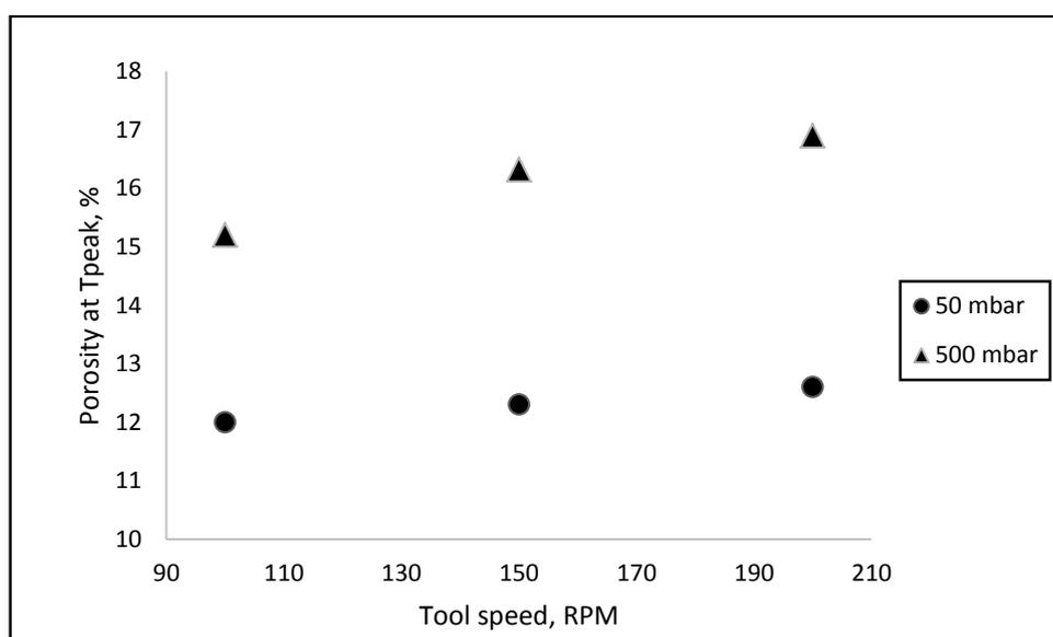
Fig. 5: Comparison of porosity at tPEAK for different pressure
