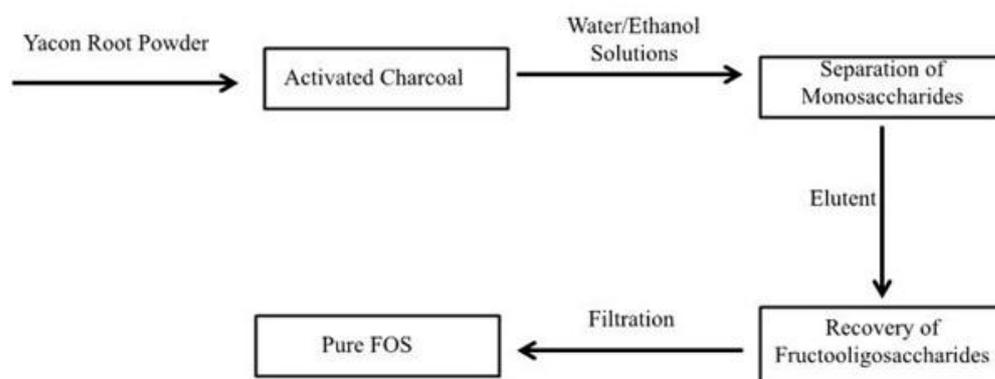
Fig. 1: Schematic process for the separation of fructooligosaccharides from yacon root
