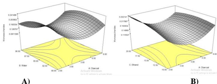
The next stage of separation was FOS from absorbed activated charcoal using more concentration of water/ethanol (v/v) elutents than first stage of separation process. From the optimal study in figure 2D showed the effect of interaction between charcoal and water. It displayed when water level increases FOS concentration was recovered up to 0.157
