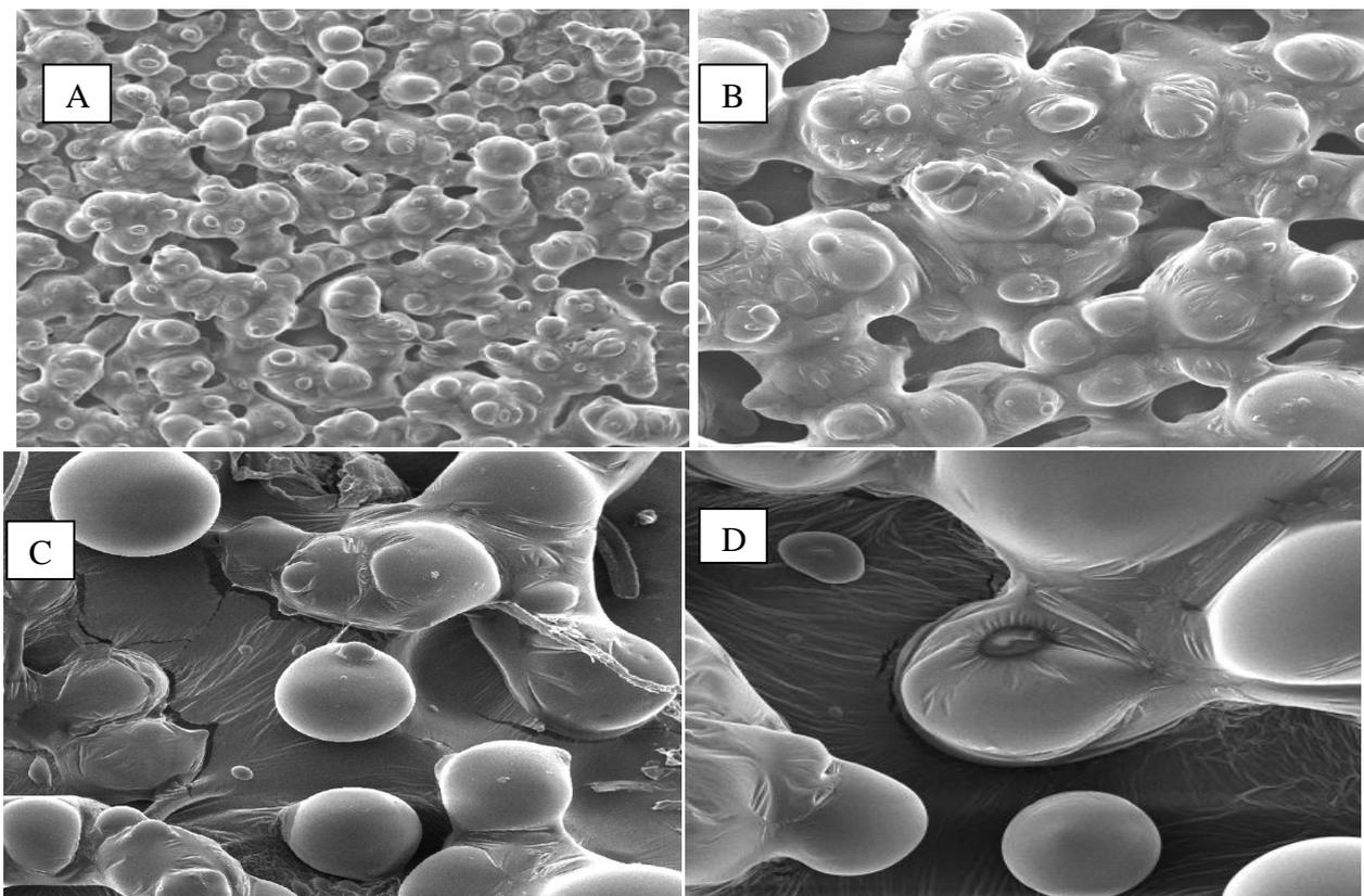
Fig. 2: SEM image for Fructooligosaccharides from yacon root powder, image A and B are commercial FOS with magnification of  $\times 250$  and  $\times 500$ . Image C was yacon FOS under magnification  $\times 500$ . Image D was yacon FOS with magnification  $\times 1000$  to view as single compound for observation after freeze-dried.
