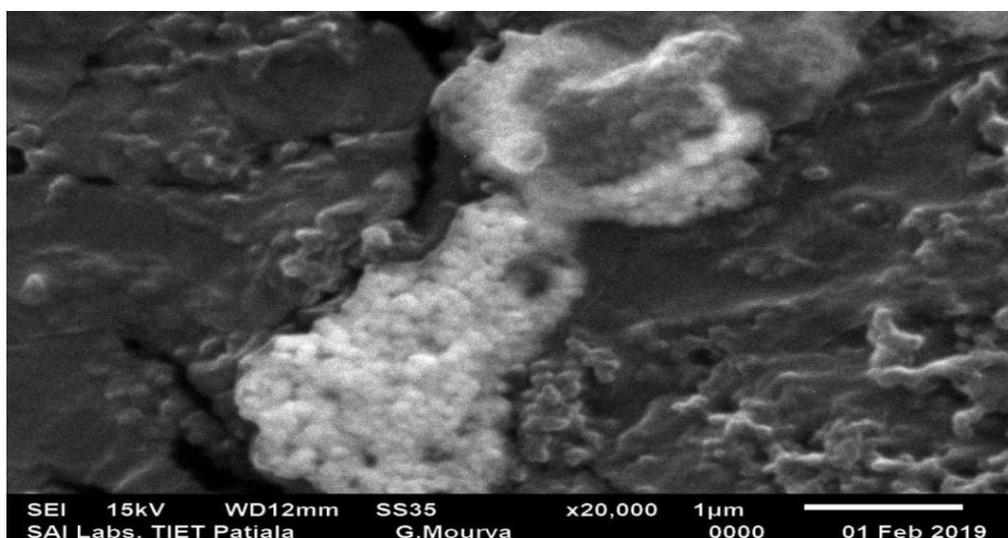
**Fig. 2:** SEM image of silver nanoparticles from *Datura metel* leaves extract
