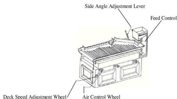
**Fig. 2. Specific Gravity Separator**
