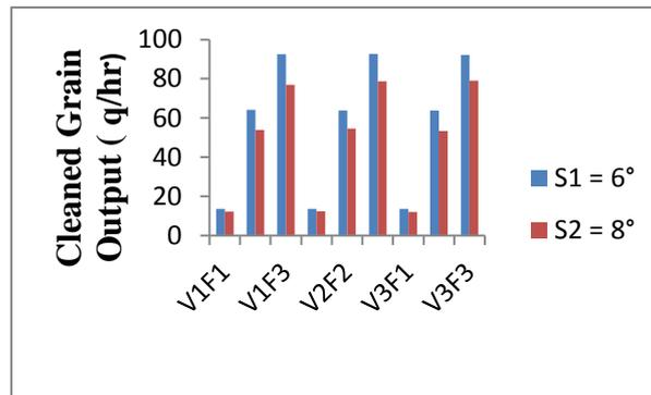
Fig. 8. Effect of screen slope on cleaned grain output for flat screen grain pre- cleaner.
