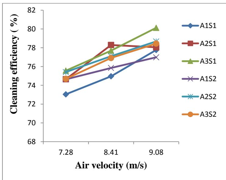
**Fig. 5. Effect of air velocity on cleaning efficiency as affected by screen effective surface area, screen slope and feed rate for flat screen grain pre cleaner.**
