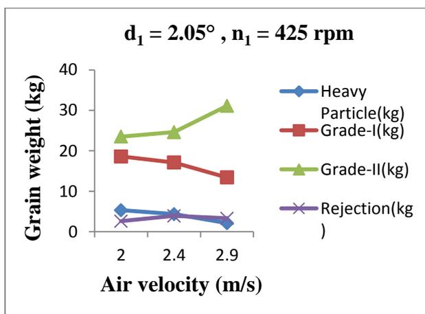
Fig. 11. Effect of Air velocity on grading quality of grain for gravity separator.
