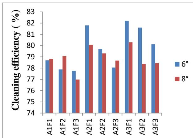
**Fig. 4. Effect of screen slope on cleaning efficiency (%) for flat screen grain pre-cleaner.**
