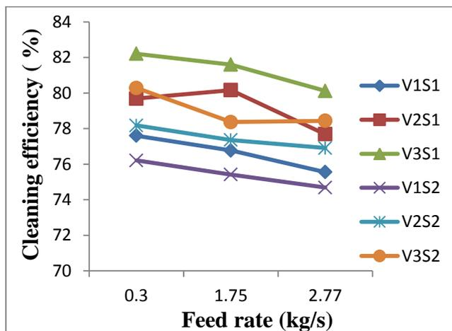
Fig. 6. Effect of feed rate on cleaning efficiency as affected by different air velocity, screen slope and screen effective surface area for flat screen pre-cleaner.
