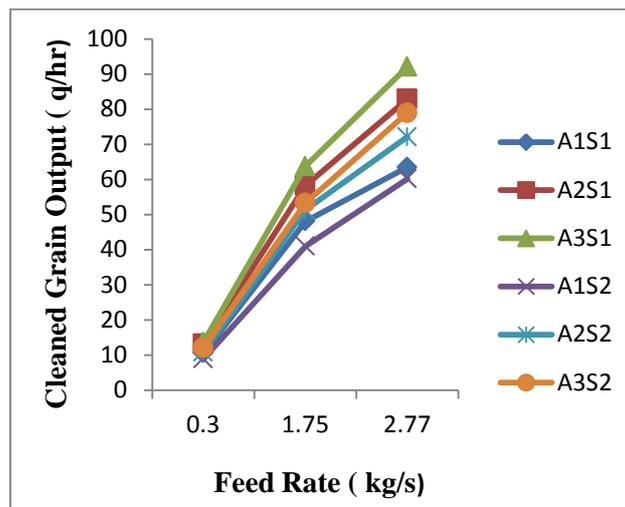
**Fig. 10. Effect of feed rate on cleaned grain output as affected by different screen effective surface area, screen slope and air velocity for flat screen grain pre- cleaner.**
