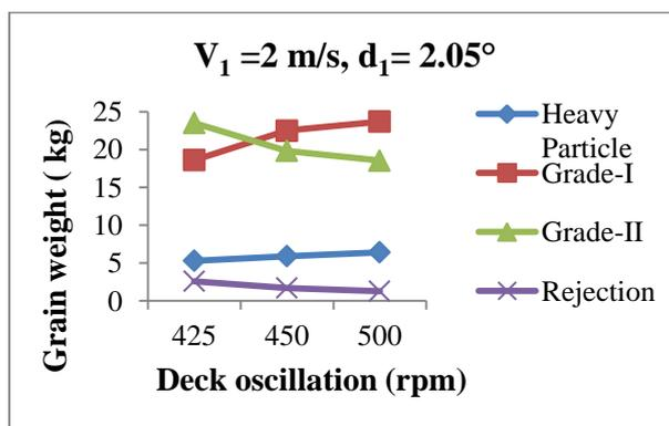
Fig. 12. Effect of deck oscillation on grading quality of grain for gravity separator.
