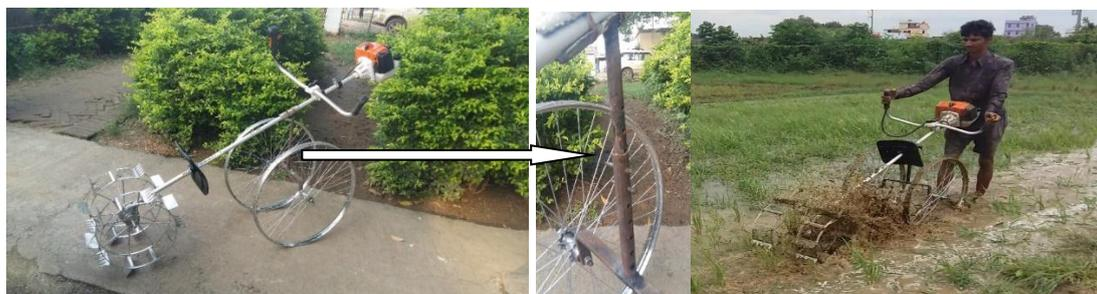
First modification to reduce vibration on body and operation at field
