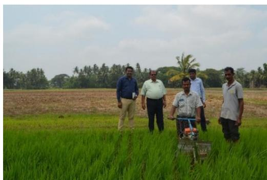
Second modified weeder to reduce vibration and maintain in line and in operation at field
