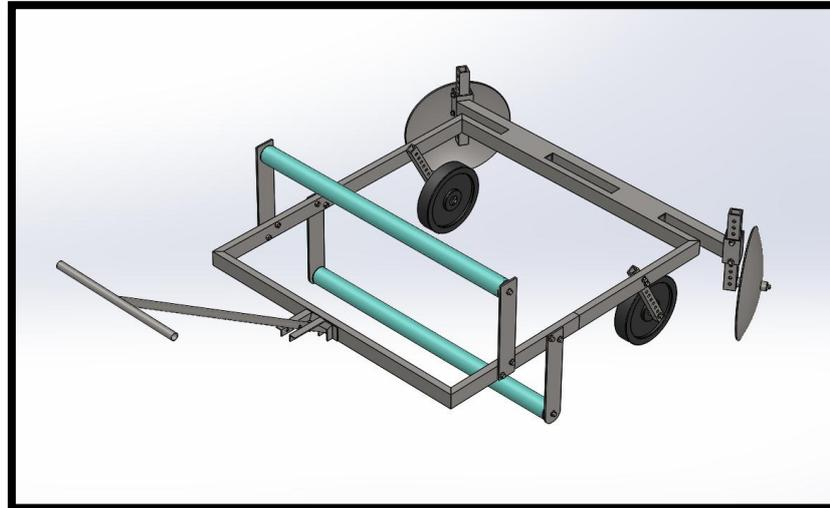
1. Handle 2. Hitching Unit, 3. Mulch Laying Unit, 4. Main Frame, 5. Press Wheel, 6. Earthing Unit
