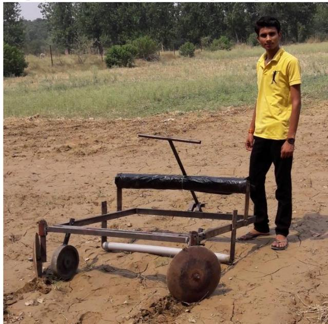
View of developed manual operated plastic mulch laying machine
