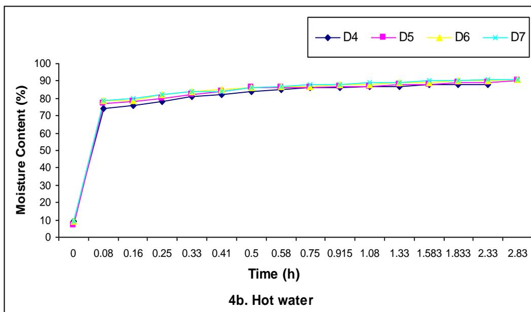
Figure 4: Effect of cabinet air drying temperatures on moisture uptake pattern of okra pieces
