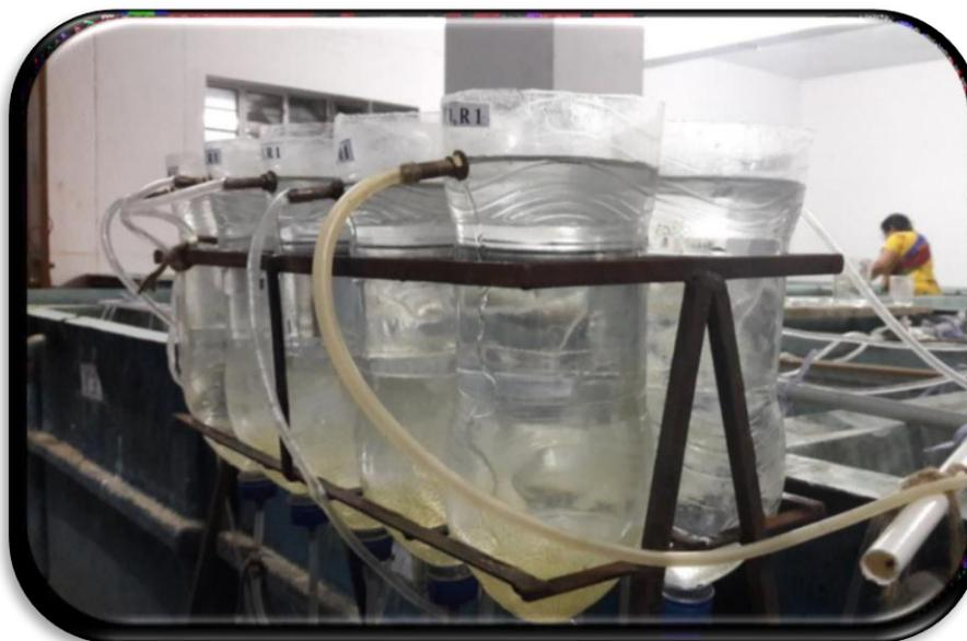
**Plate 1: Simple hatching device fabricated for egg incubation**
