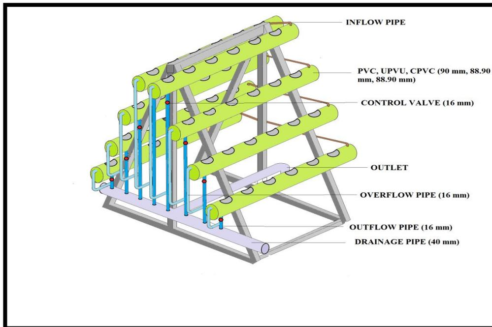
Fig. 1: Isometric view of a shaped frame hydroponic structure
