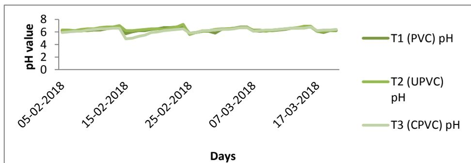
Fig. 5: pH values of hydroponic solution after changing the nutrient solution in a shaped frame structure under different treatment
