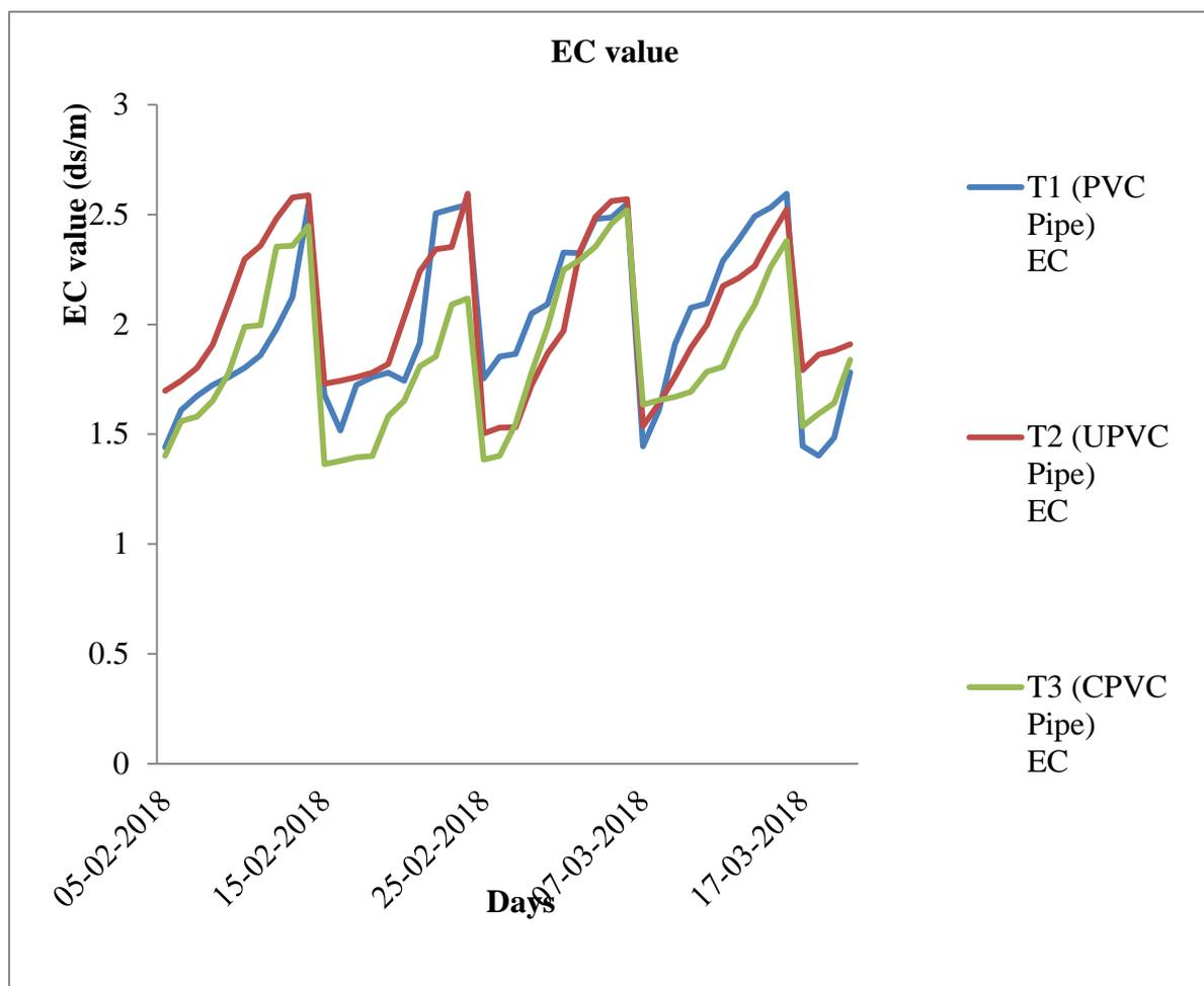
**Fig. 6: Values of EC of hydroponic solution after changing the nutrient solution under different treatment in a shaped frame structure**
