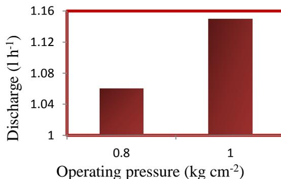
**Fig. 1: Discharge variation under different operating pressure**
