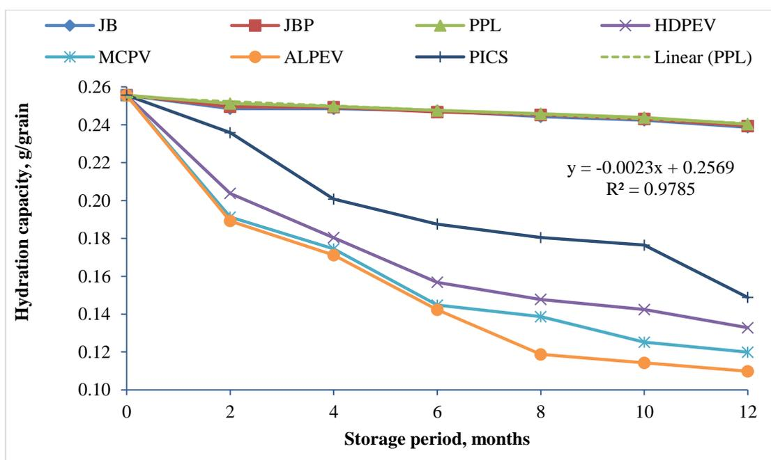
Fig. 3: Effect of different packaging materials on hydration capacity of chickpea grain
