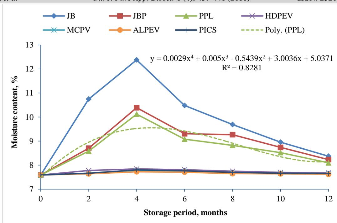
Fig. 1: Effect of different packaging materials on moisture content of chickpea grain
