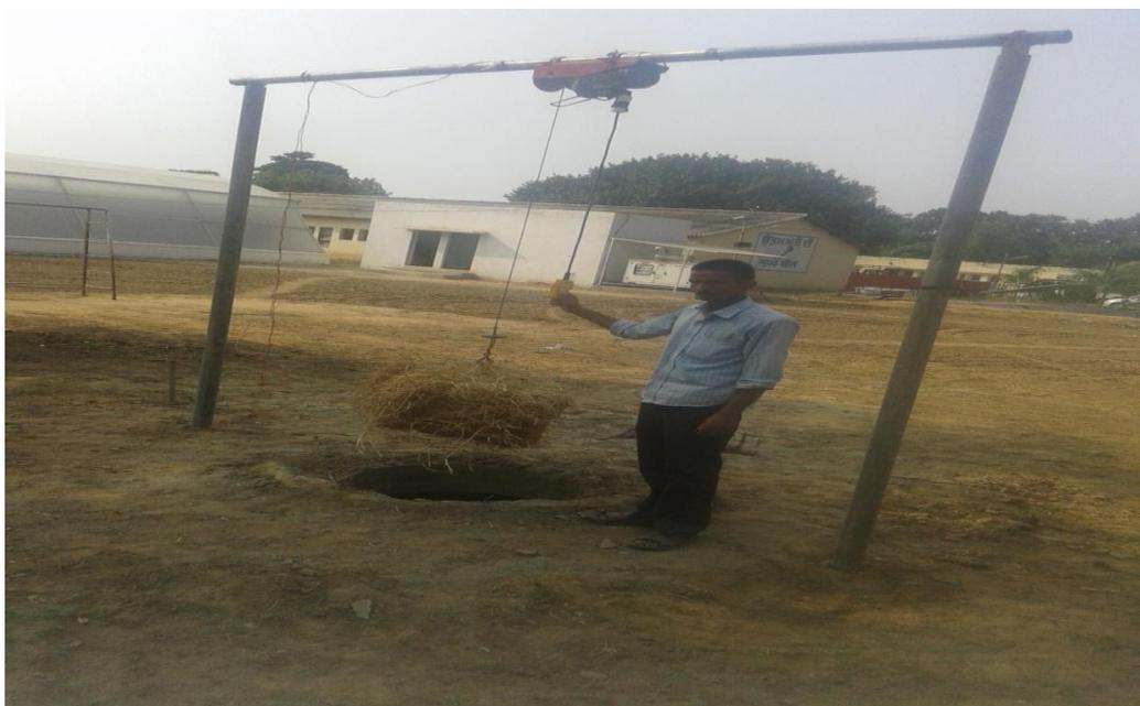
Fig. 5: Bales lifted by Semi-automatic solid bio-digested slurry lifting machine
