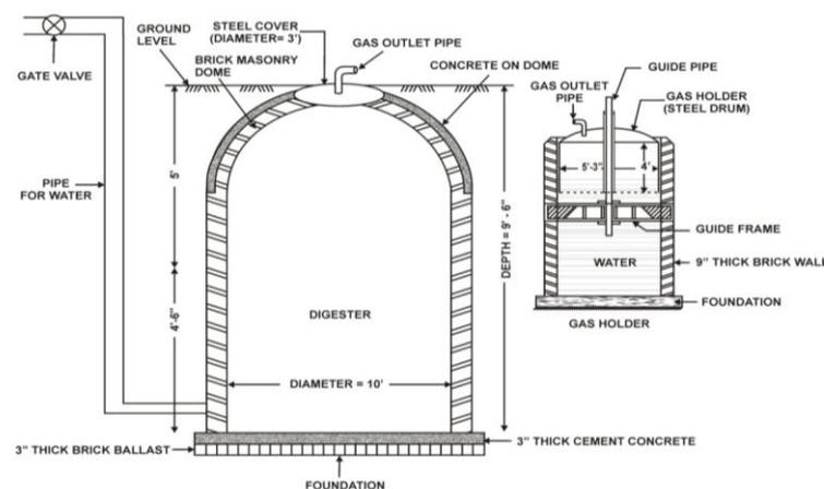
**Fig. 1: Dimensions of Dry Fermentation Biogas Plant**
