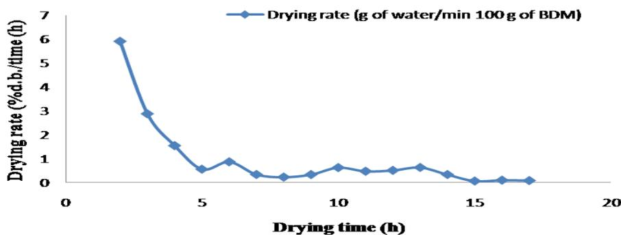
Fig. 2: Variation in drying rate with drying time (min): sun drying
