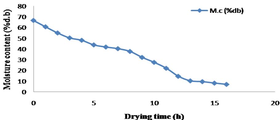
Fig. 1: Variation in moisture content (%d.b.) with drying time (min): sun drying
