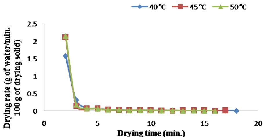
Fig. 4: Variation in drying rate with drying time (min): Fluidized bed drying
