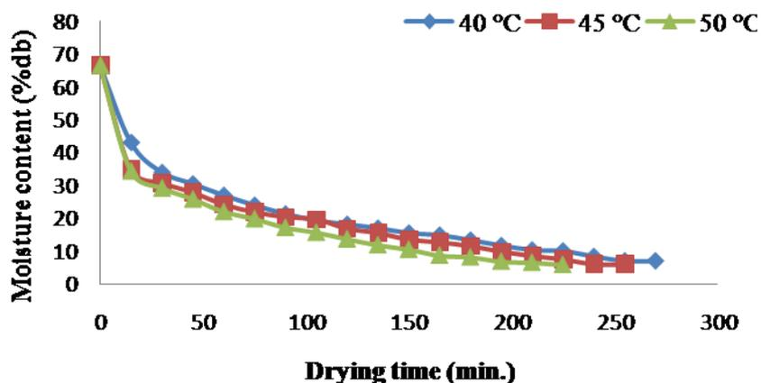
Fig. 3: Variation in moisture content (%d.b.) with drying time (min): fluidized bed drying
