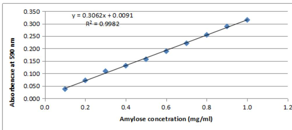
Fig. 2: Standard graph of amylose solution using antrone reagent
