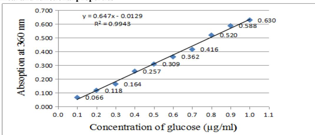
Fig. 1: Standard graph of glucose solution using anthrone reagent
