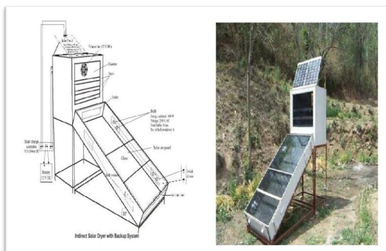
Fig. 8: a) Schematic view b) Pictorial view of forced circulation solar dryer for hill products
