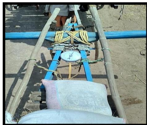
Fig. 1: Measurement of draft
