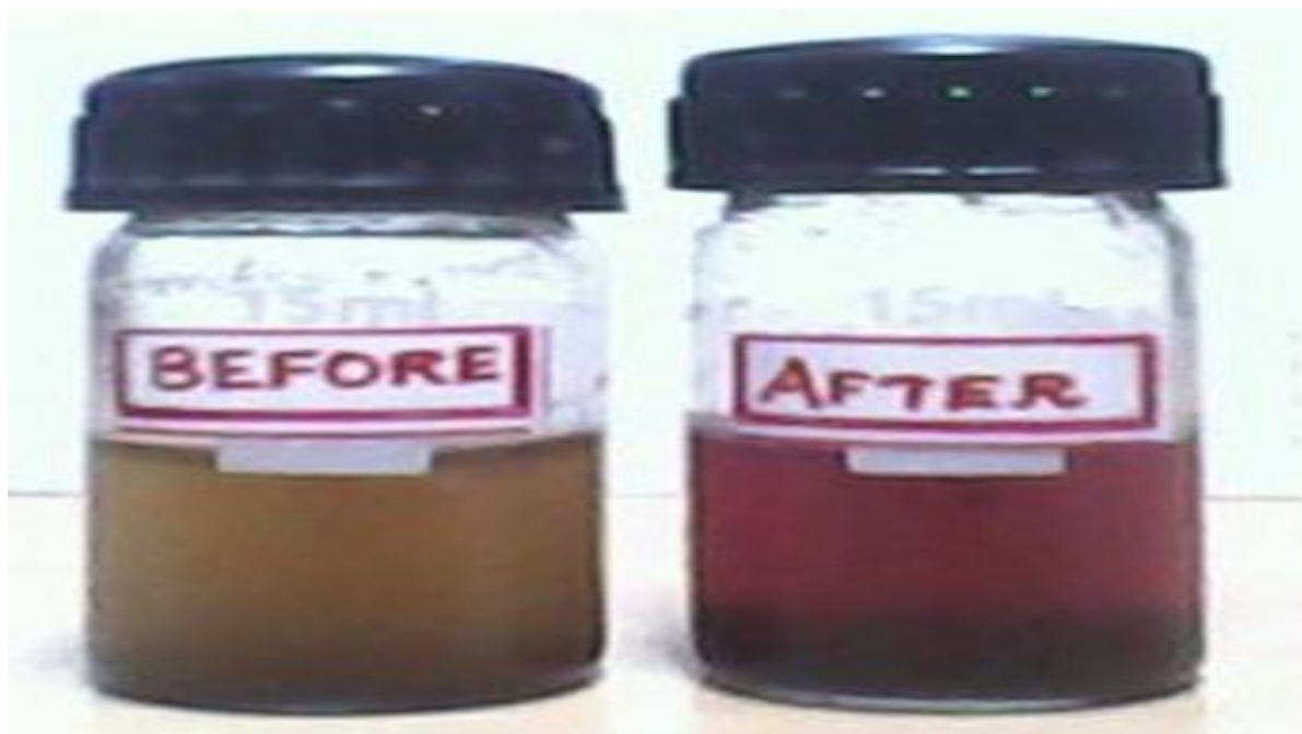
Plate 7: (A) The biomass of S. myriocystum with gold ions at the beginning of the reaction (B) The colour change of the medium to Ruby red color after incubation
