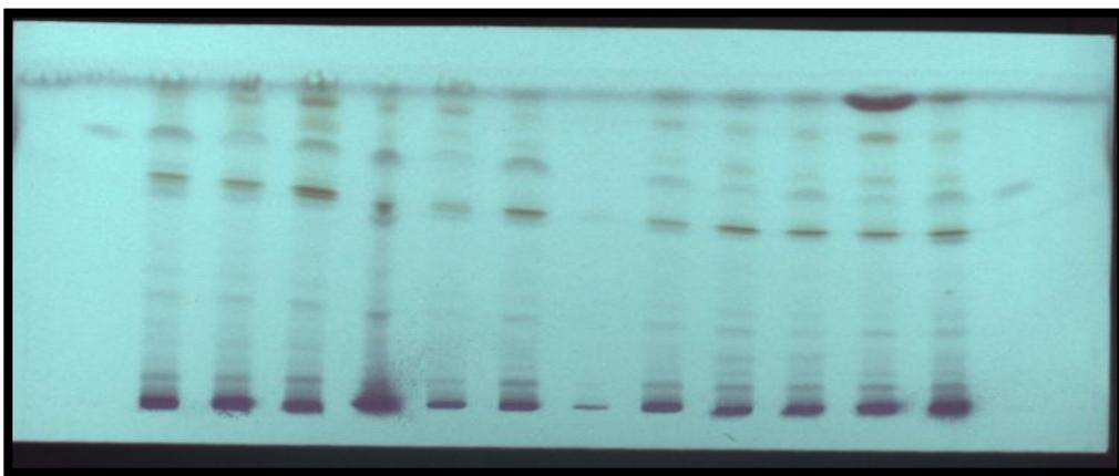
**Plate No. 2 [UV light] Picture of bands in silica gel plate after passing through Gibb's reagent, dry air and ammonia vapour successively under ultra-violet light**
