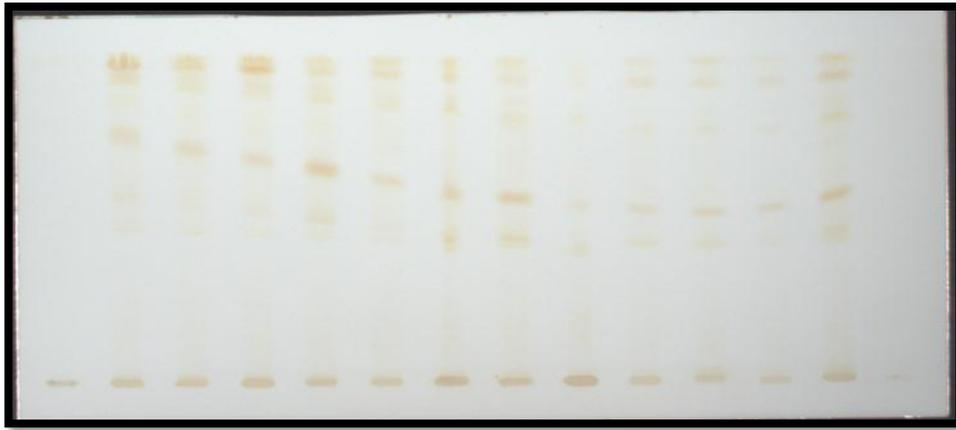
**Plate No.1[White light] Picture of bands in silica gel plate after dipping through Gibb's reagent under monochromatic light**
